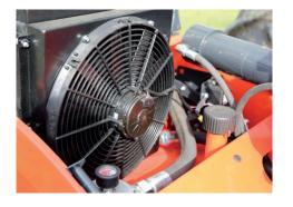
Oversized oil cooler: 12 kW as standard, offers constant power and protection of hydraulic components.
