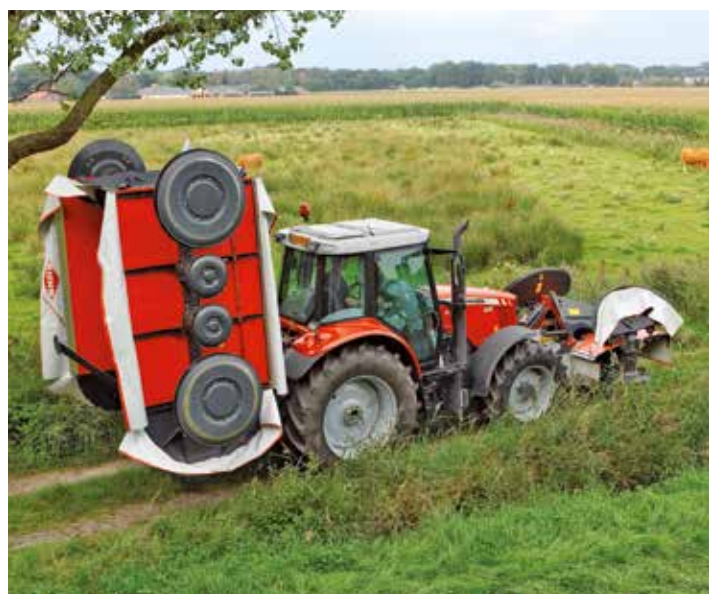
For a road transport width of less than 3.00 m, the mower units are swung upwards using hydraulic cylinders
