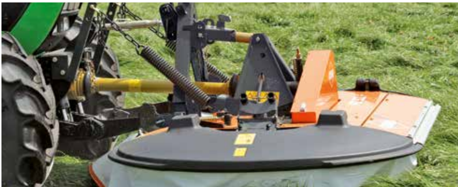
PENDEFLEX pendulum headstock
