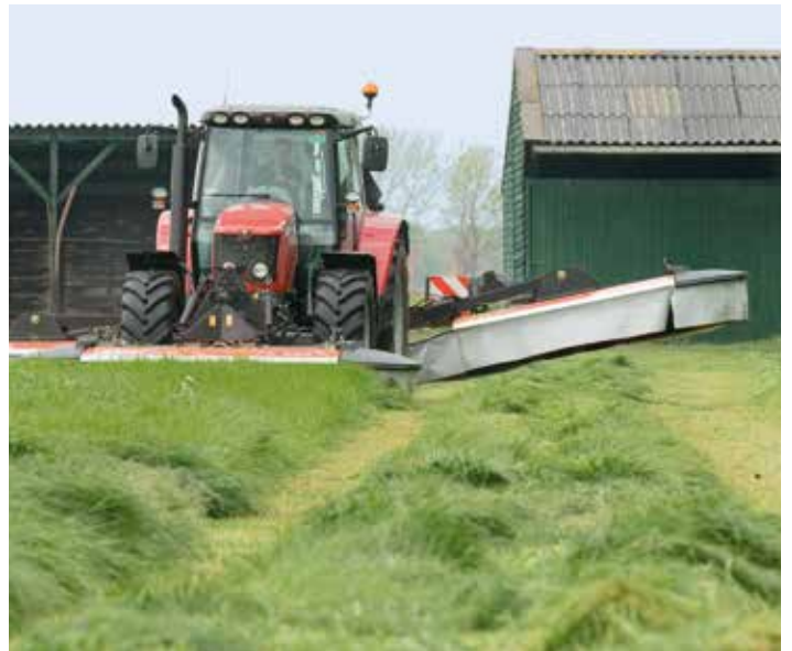
Independent lifting. The PZ 960 drum mower rear combination is equipped with a functional hydraulic valve as standard
