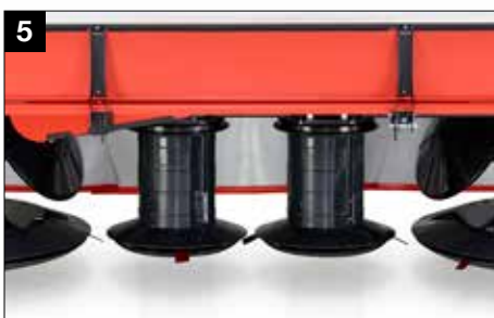
Standard swath discs securing a narrow swath
