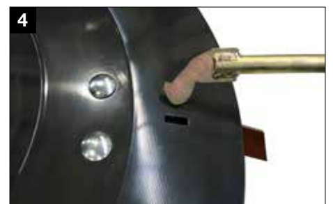
Knife changing system with special tool and knife holder
