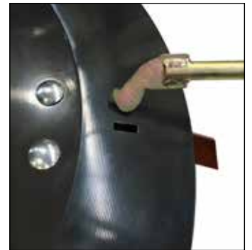
Quick knife exchange system
