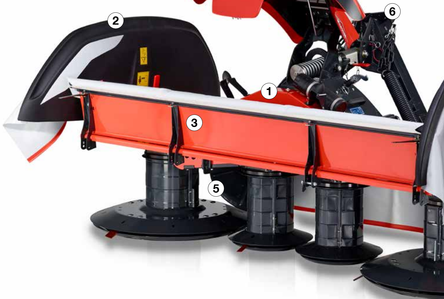
V-belt drive with large 40 mm bearings & strong mainframe
