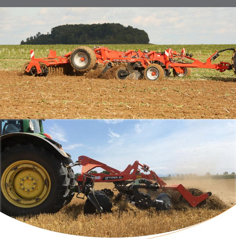
OPTIMER XL: intensive mixing at high speeds with 620 mm diameter discs.
