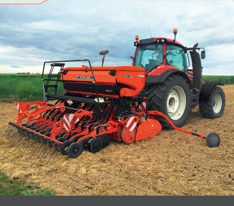
The mechanical seed drill range SITERA 3010/3020/3030 now counts the additional models SITERA 3010/3020/3030 e with electrical distribution drive. The machines are equipped with an electrical motor on the right hand side and a radar sensor for the speed signal. You can choose between the VT30 terminal, the ISOBUS version compatible with the CCI 800 or 1200 or another ISOBUS terminal.
