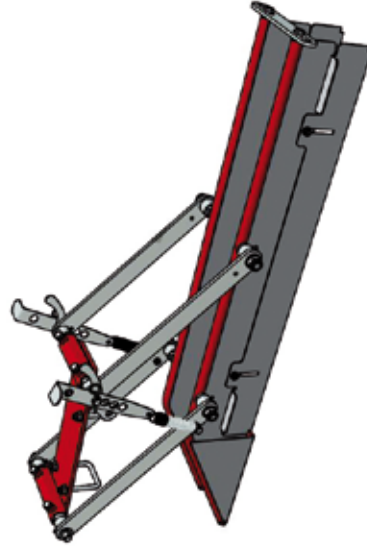
Leaf protector mounted in parallelogram (width adjustable)
